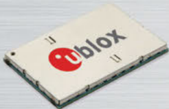
TOBY-L1/L2 LTE modules 24.8 x 35.6 x 2.6 mm
