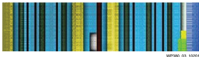
Figure 3: FPGA Die Slice Optimized for Stacked Silicon Integration
